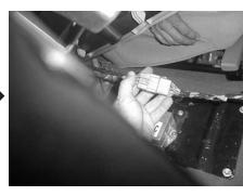
**STEP 10:** Tilt the console up from the rear. This will expose another harness with a white plug, disconnect.
